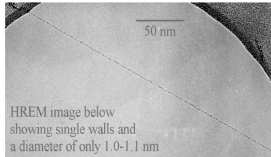
Figure 3. TEM image of a single-walled carbon nanotube showing the long aspect ratio of the tube and the potential for asbestos-like behavior.
