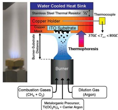
**Figure.** A schematic diagram of an aerosol flame reactor for making TiO<sub>2</sub> nanostructures.
